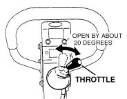
Figure 9. Throttle Lever (Start)
